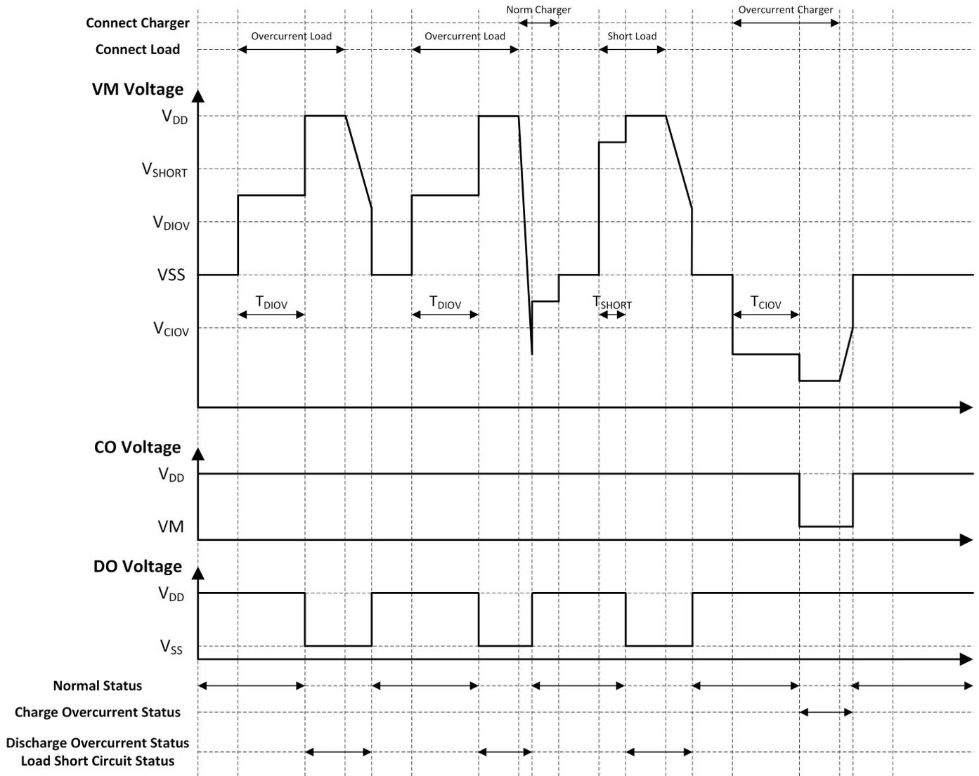
**Note1:** As the delay of exiting Charge Overcurrent/Discharge Overcurrent/Load Short Status is very short, the delay is not marked in the Figure.
