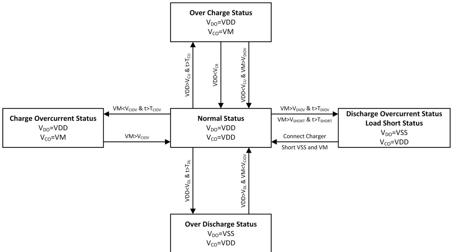
Note: VM and  $V_{CI0V}$  are signed digits. For example: If  $VM = -200mV$  and  $V_{CI0V} = -100mV$ , that is  $VM < V_{CI0V}$ .
